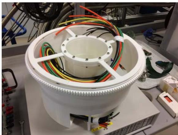
Figure 4: Image showing a prototype of the cable management mechanism produced to evaluate its effectiveness.
