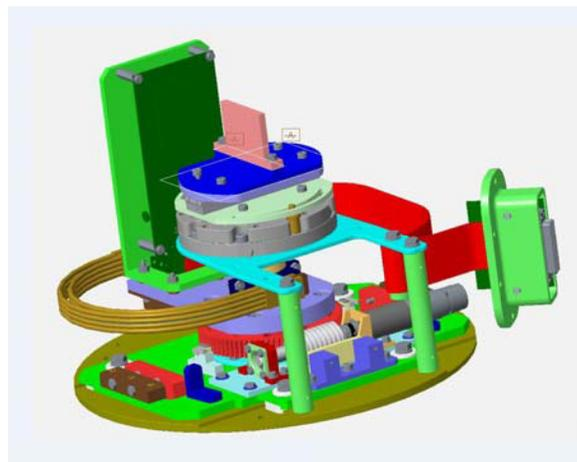
Figure 5: CAD model of the mechanism located inside the main vacuum chamber showing the detector mounted on its rotary stage with thermal and electrical connections. The face of the detector is approximately at a 100mm radius from its axis of rotation.
