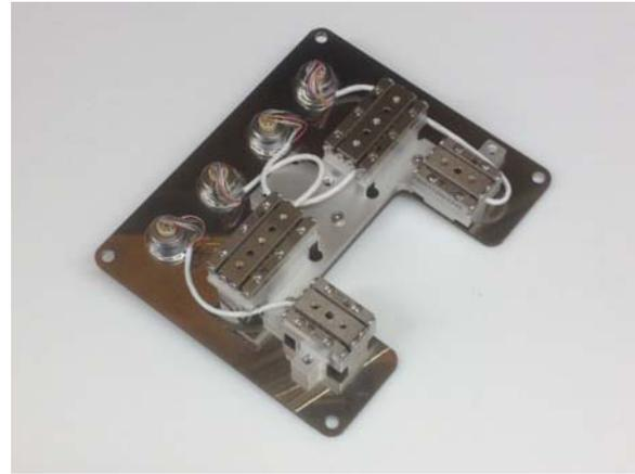
Figure 3: An example of a compact in-air slits assembly designed in collaboration with SmarAct GmbH. Stages shown have ranges of 12mm and 20mm with sub-micron resolution.
