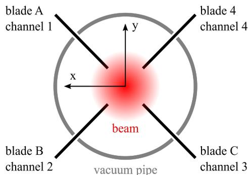
Figure 1: XBPM schematics.
