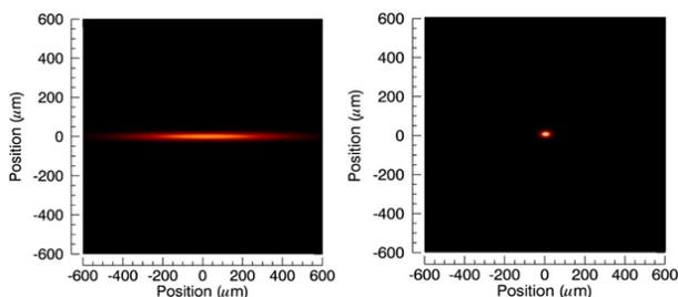
Figure 1: APS electron beam before and after upgrade.
