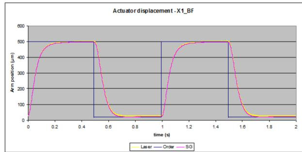
Figure 10: SG versus Laser Interferometer.
