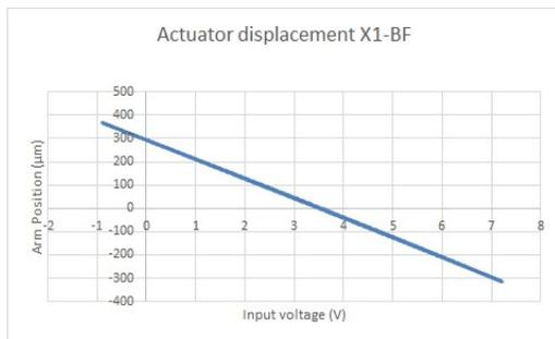
Figure 9: Mechanism displacement in closed loop.
