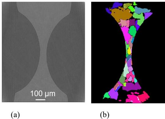
Figure 3: a) A classical transmission radiography of a single lens. b) A differential contrast tomography. The refractive lens is produced by cold-punching. Grain sizes are revealed. The quick deformation produced a high temperature rise of the material and then a dynamic recrystallization- Courtesy W. Ludwig-ESRF-ID11.
