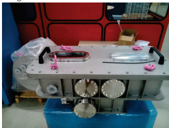
vacuum tank for lens system
