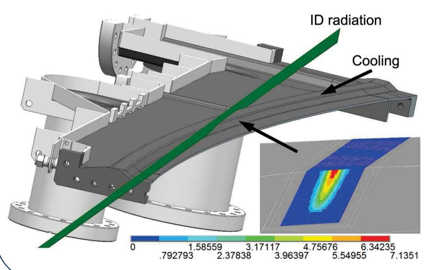
Schematic cross-sectional view of standard dipole vacuum chamber, displaying the lower longitudinal cooling channel and ID radiation interference for vertical mode polarization. The footprint is in W/mm<sup>2</sup>.
