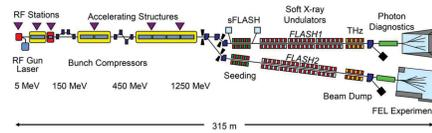
Figure 1: Schematic overview of the FLASH I and FLASH II accelerators
