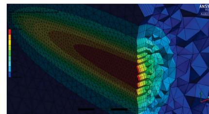
Figure 9: Final FEA result, peak temperature of 102°C in red in the middle.
