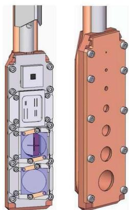
Figure 7: Diagnostic paddle (left) and aperture paddle (right). Aluminum support rod and copper cooling pipes visible on top.
