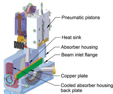
Figure 8: Mechanical concept. Absorber housing cut open.
