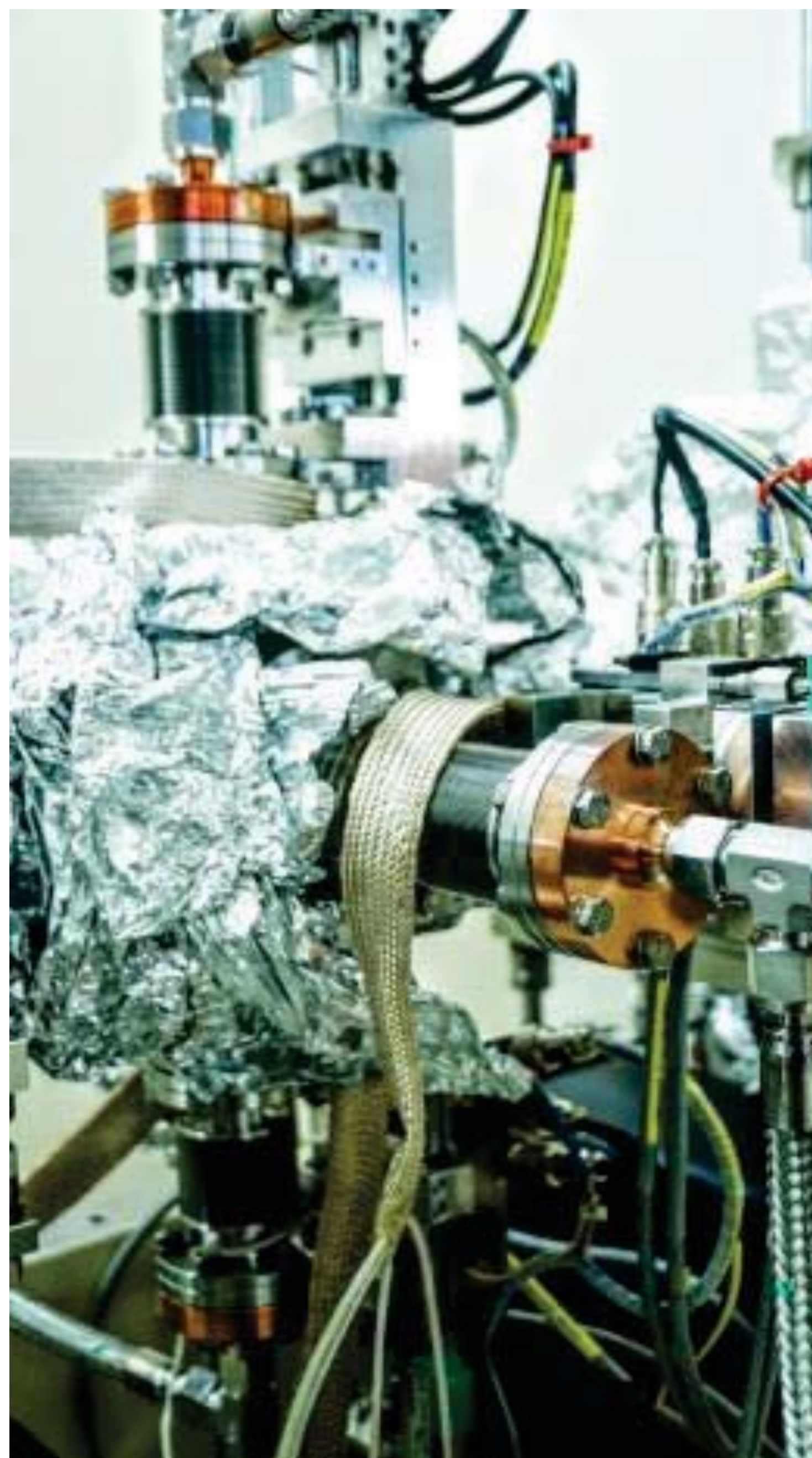
CuCrZr slits in TPS front end 24
