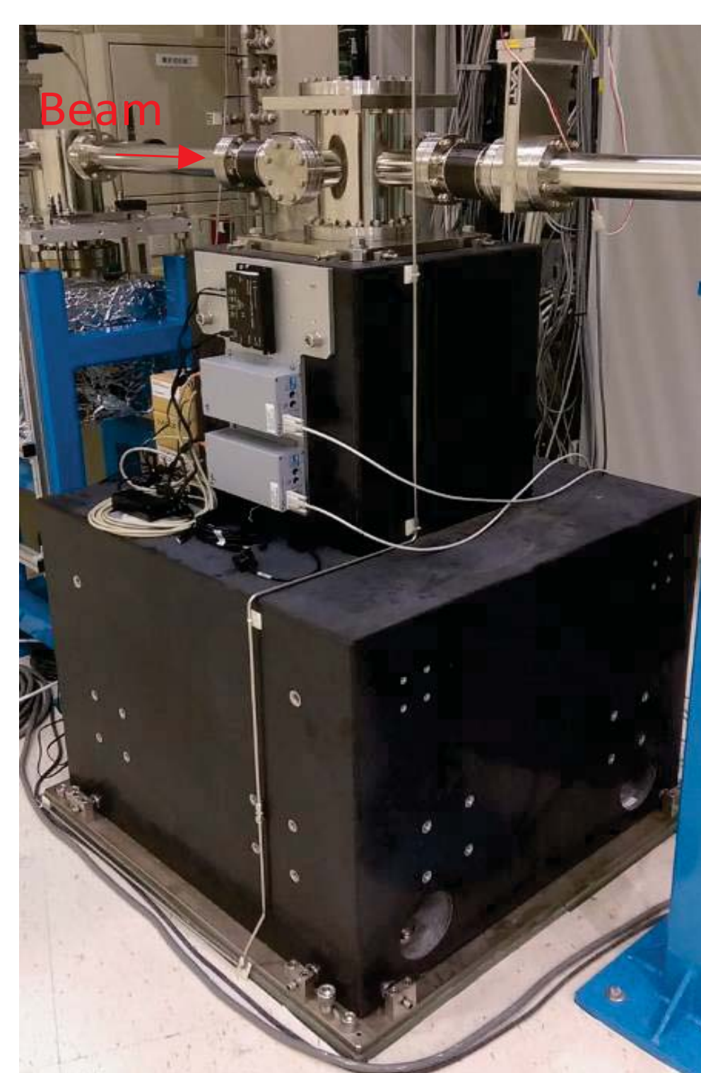
Figure 2: On-site view of secondary source slits installed in the Coherent X-ray Scattering beamline at TPS.
