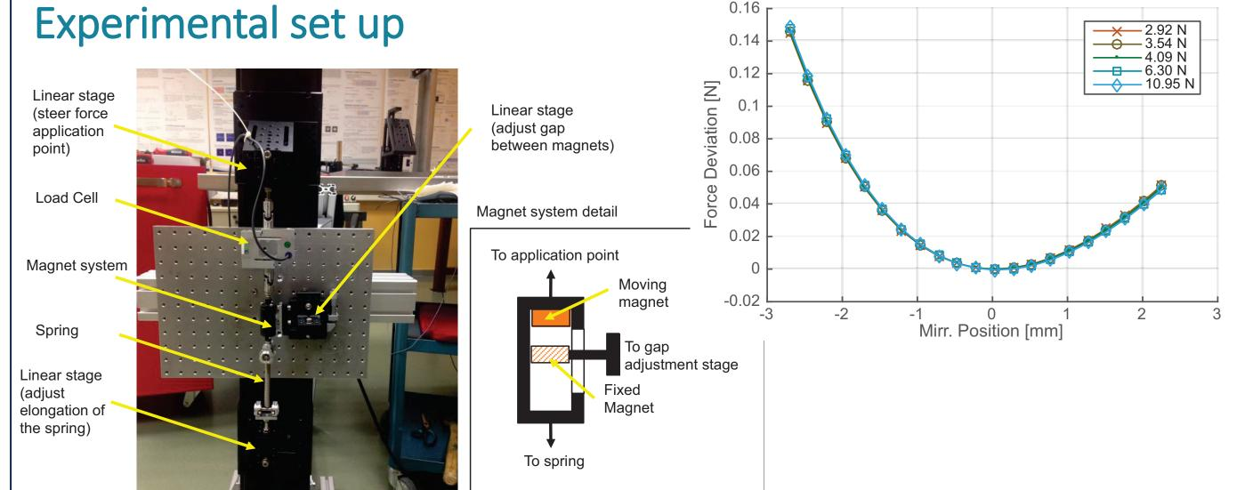
The flexure torque has a linear dependence on the angle while the magnetic force is given by an inverse law. The sum of the three torques is zero around its nominal position and it is stable in an angle range around this point where the torque is independent of the angle.
