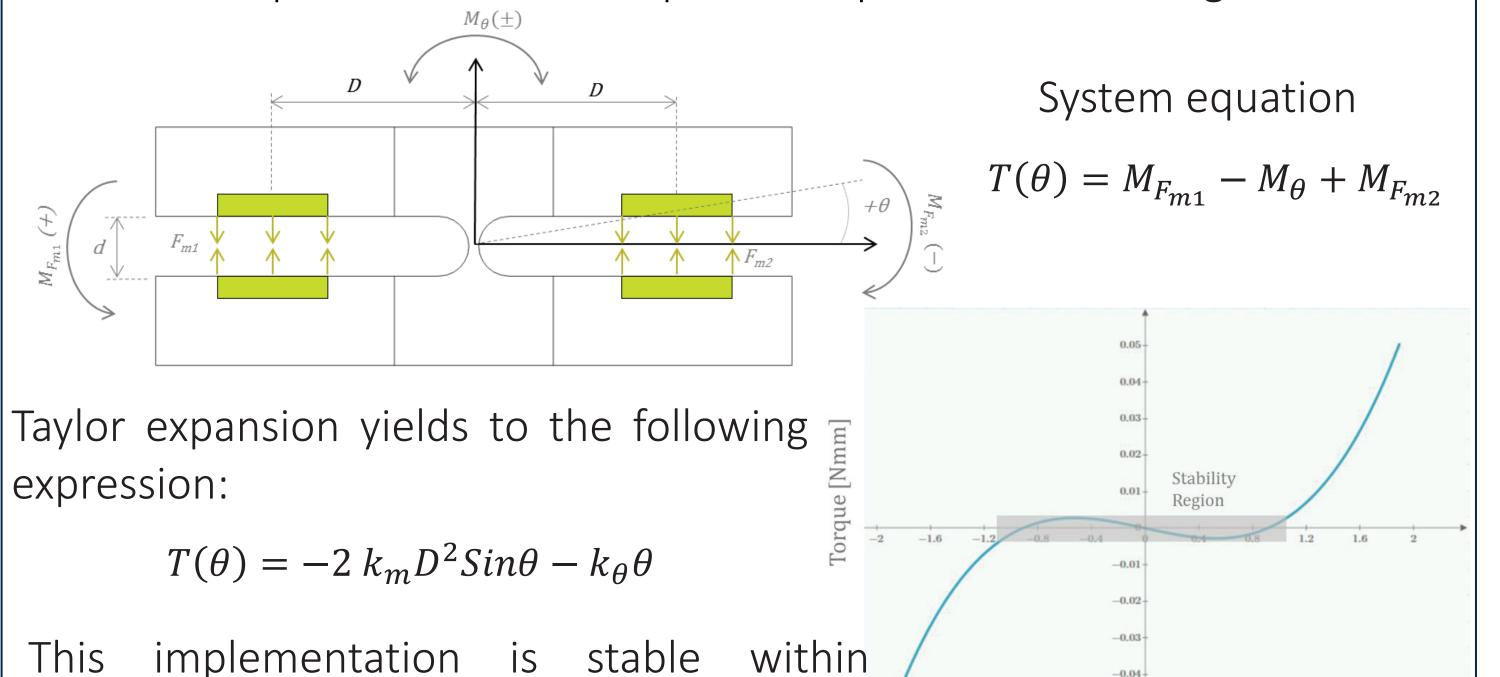
The stabilization is the minimum in which there is only a variation of 0.02 N for a range about 2.3 mm and is independent of the nominal ES Patent: **P201630506** force.
