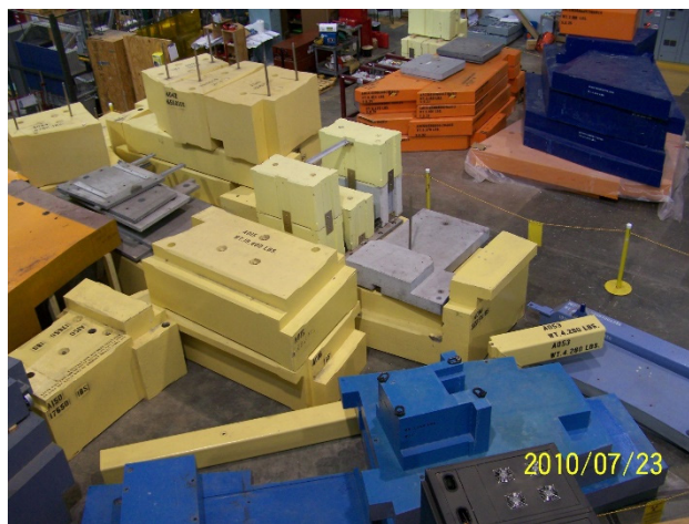
Figure 1: Neutron shielding from the Spallation Neutron Source, Oak Ridge National Laboratory, USA.
