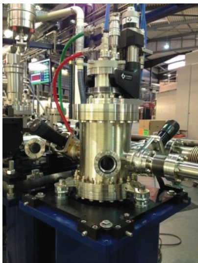
Figure 3: Complete chopper unit.
