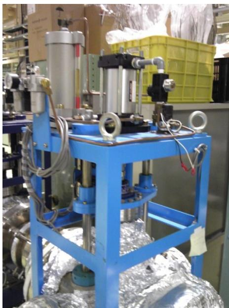
Figure 9: Old Safety Shutter: Oil-Hydraulic Cylinder.
