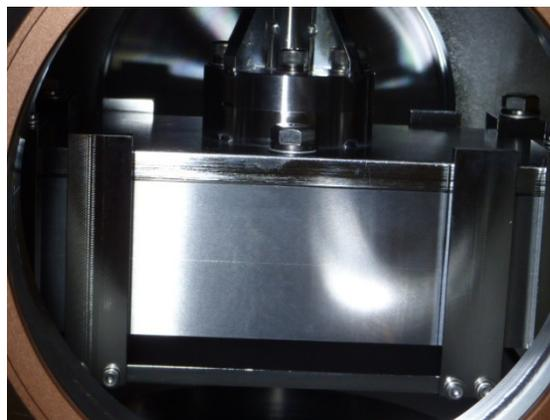
Figure 11: New Safety Shutter: 250-mm Thick Tungsten Block.
