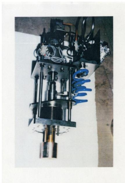
Figure 4: Photon Shutter for Undulator BL Front End (Old Type).
