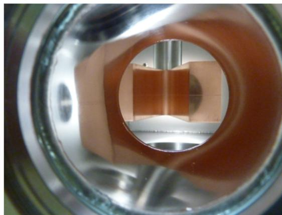
Figure 7: Photon Shutter for Multi-Pole Wiggler and Long Undulator BL Front End (New Type).
