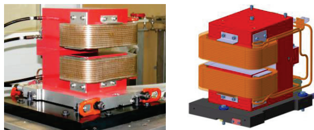
Figure 4: 3D model (right) and fabricated chicane dipole (left).
