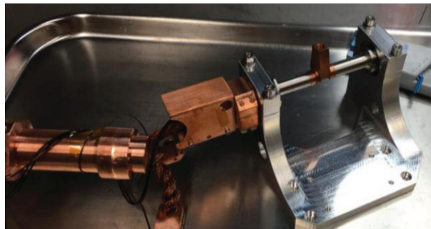
Figure 4: Apparatus used for the preliminary thermal tests. The copper hardware on the left connects to the cryostat (not shown) and an aluminium yoke holds the stainless steel-glidcop sample holder to complete the trunnion assembly.
