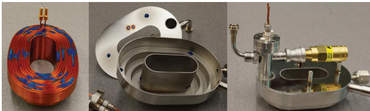
Figure 2: Our prototype wound coil (left), stainless steel coil can prior to final assembly (center), and the final assembled prototype coil-can assembly (right).
