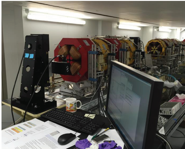
Figure 4: Stretched wire measurement of magnet groups.
