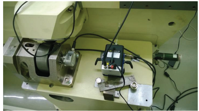
Figure 6: A shaker to simulate the vibration source.
