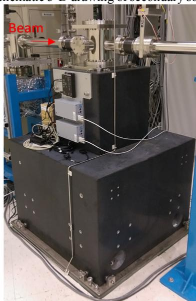
Figure 2: On-site view of secondary source slits installed in the Coherent X-ray Scattering beamline at TPS.
