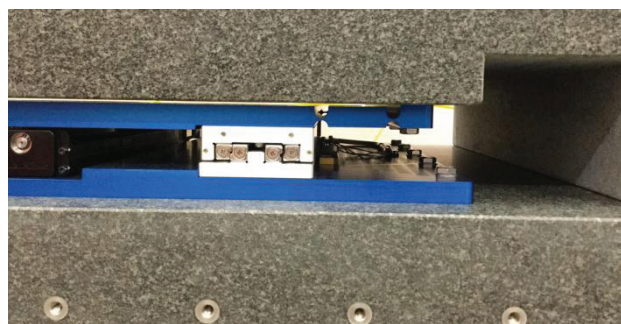
Figure 14: X-axis actuator and guidance for air bearing.
