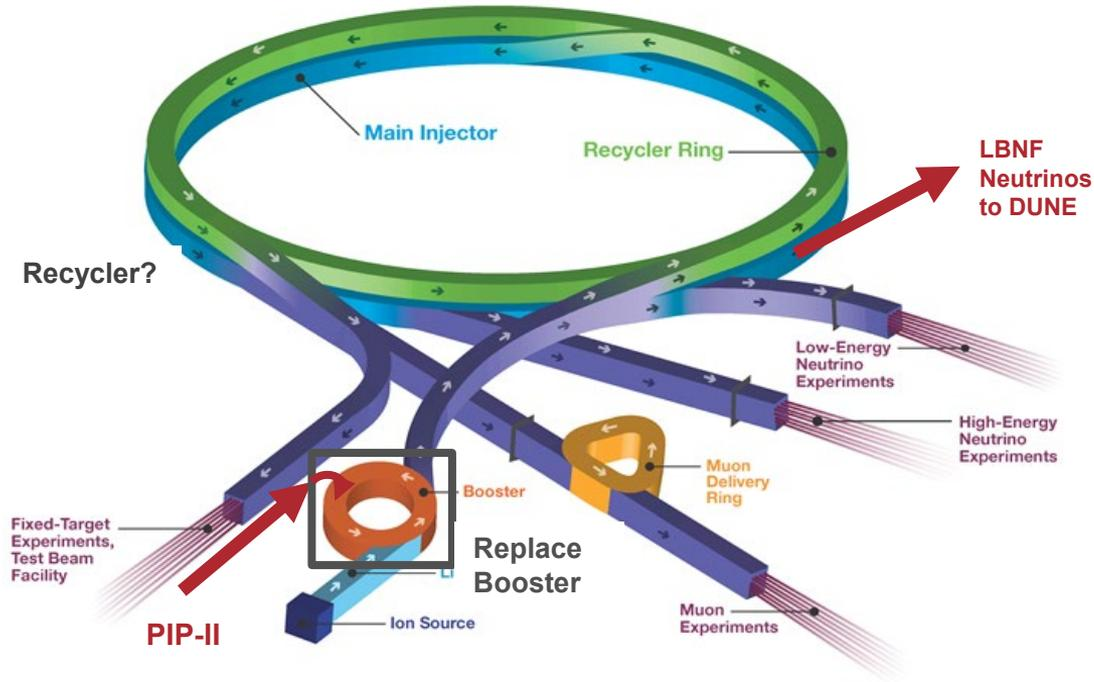
After PIP-II goes online, booster will be the bottleneck for proton power on target for LBNF/DUNE
