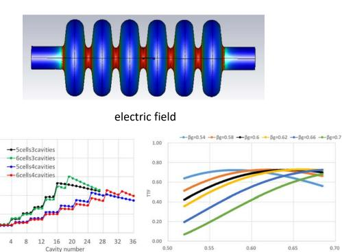
6 cells per cavity, 3 cavities per cryomodule
