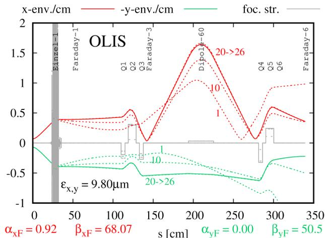
Figure 3: TRANSOPTR 2rms envelope optimization. Optimum Einzel lens ( $s \sim 25\text{cm}$ ) and 5 quadrupoles set points are found to produce the requested Twiss parameter match at the simulation end. After 26 iterations, the optimum set points are returned from the optimizer. All files have been automatically generated from an element position repository. Units of  $\beta$  are cm/rad.
