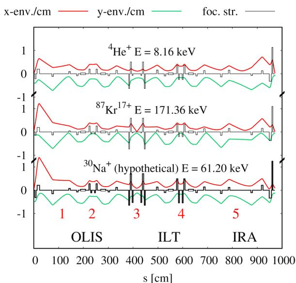
Figure 4: TRANSOPTR sequentially finds tunes in under 60 seconds, by breaking up long sequences into sub-segments with 4-6 optimization variables. This allows us to compute full linac tunes from first principles for on-line tuning. All files autogenerated.
