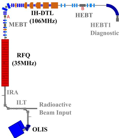
Figure 1: Schematic representation of the ISAC linac at TRIUMF. A & B are stripping foil locations
