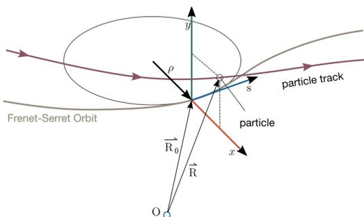
Figure 2: Sliding Frenet-Serret coordinates.
