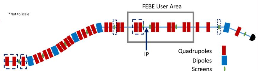
Fig. 1 – A latter section of the FEBE CLARA beamline. Quadrupoles varied and screens used in simulations are indicated.
