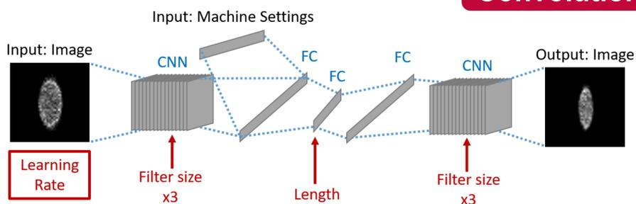
Fig. 2 – The model structure of the full tunable CNN. Tuned parameters are in red, model components in blue. CNN = Convolutional Neural Network; FC = Fully Connected.
