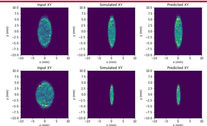
Fig. 3 – Example inputs, simulated outputs, and predicted outputs for the two models. Top: Pre-IP method. Input from FEBE CLARA transfer arc, output at IP. Bottom: Post-IP method. Input from FEBE CLARA beam dump, output at IP.
