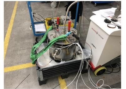
Figure 5: Evacuation of the cavity at room temperature.
