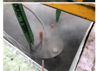
Figure 7: The cavity was installed vertically in a tub filled with LN<sub>2</sub>.
