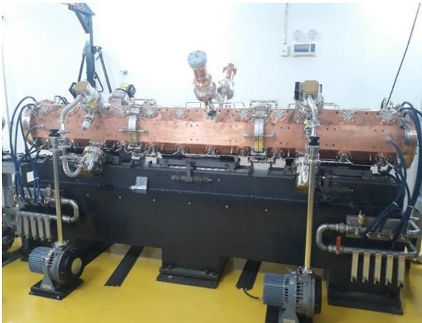
Figure 2. Fabricated RFQ
