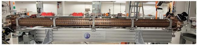
Figure 2: TDC structure installed in the beamline. The electron beam travels from left to right.
