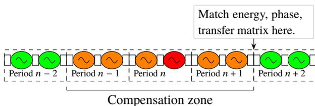
Figure 1: Scheme of a failed cavity (red) at the lattice period  $n$ . The  $k = 5$  neighboring cavities (orange) compensate for the fault; cavity settings outside of the compensating zone remain in nominal tuning (green).
