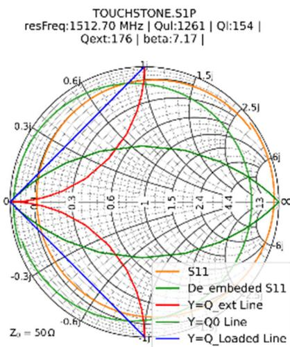
Figure 7: Qs from model and low level 'measurements'.
