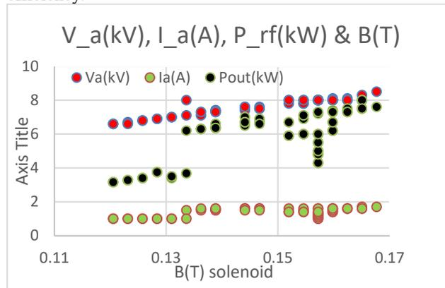
Figure 10: RF power, anode voltage and current vs. magnet field.
