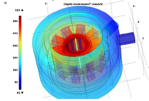
Figure 5: Anode body and water-cooling T distributions.
