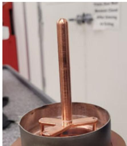
Figure 2b: Antenna attached to anode body.
