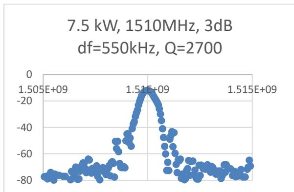
Figure 9: RF signal at 7.5 kW, single trace.
