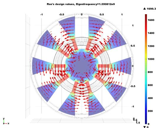
Figure 4: Electric field for pi-mode.
