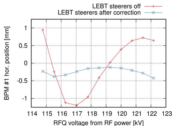
Figure 3: Oscillation of the horizontal beam position during the RFQ voltage scans, before and after correction of the trajectory in the LEBT, as measured by the first BPM in the MEBT.
