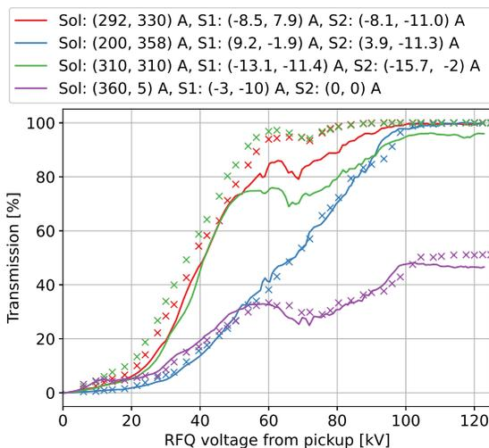
Figure 1: Beam transmission through the RFQ for different inter-vane voltages and four different LEBT configurations. The data shown as lines are measurements, the data shown as crosses are predictions by a model built upon ion source commissioning data.
