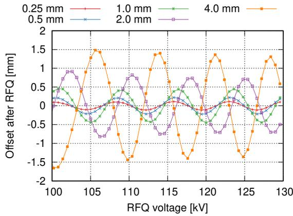
Figure 4: Model prediction of the horizontal beam offset after the RFQ as function of the RFQ inter-vane voltage in a range where transmission remains relatively constant, for different injection offsets. This was calculated using Toutatis with the first distribution shown in Fig. 2.
