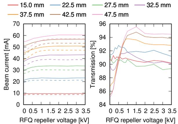
Figure 5: Impact of the voltage on the electron repeller in front of the RFQ. The beam current sent to the RFQ was changed by varying the diameter of the iris. The left plot shows the current injected (solid) into and the accelerated (dashed) current as function of the repeller voltage. The right plot shows the calculated RFQ transmission.
