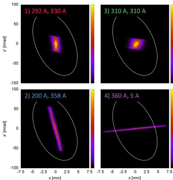
Figure 2: Transverse beam distributions at the RFQ matching plane for the different LEBT settings used to study RFQ transmission as function of inter-vane voltage in Fig. 1. The ellipses indicate the predicted zero-current acceptance.
