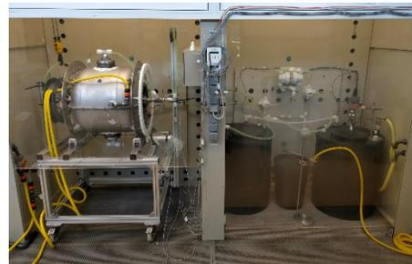
Figure 1: Rotational BCP setup at IJCLab
