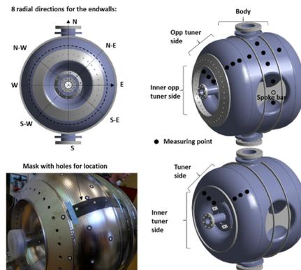
Figure 4: Thickness measurements.
