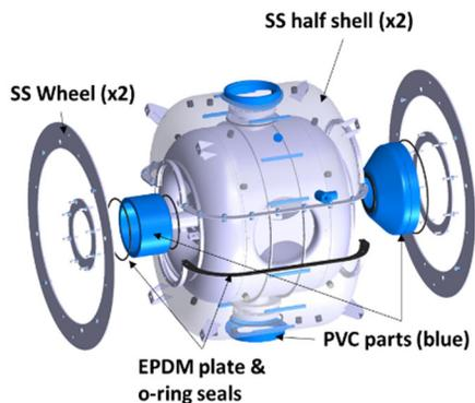
Figure 2: Dummy tank for SSR2 bare cavity
