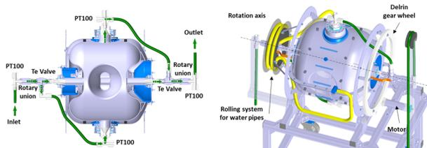
Figure 3: Acid and water circuits.
