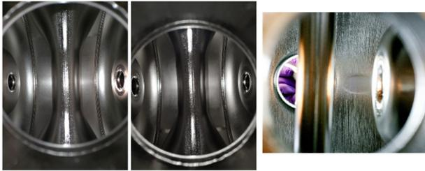
Figure 5: Surface finishing of SSR2 cavity after static BCP (Left), after rotational BCP (Center) – SSR1 cavity after static BCP (Right).
