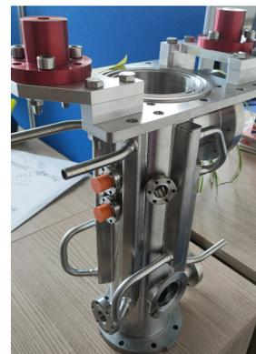
Figure 1: Quarter-wave resonator cavity prototype.
