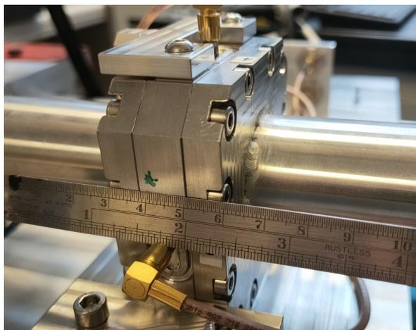
Figure 2: Button-type beam position monitor.
