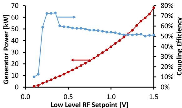
Figure 5: Generator power (red) and RF coupling efficiency (blue) as a function of input power at 3.23 MHz.
