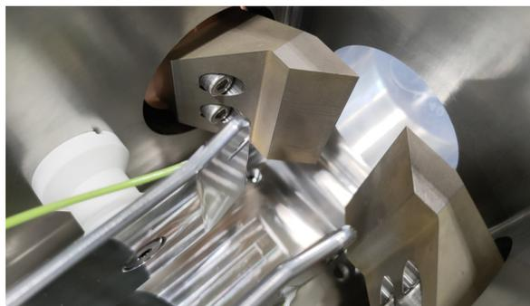
Figure 3: Chopper deflector plates and dump wedges.
