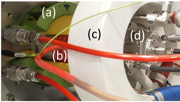
Figure 4: H<sup>-</sup> ion source. Main components: filter magnets (a), RF-coil (b), cooling jacket (c), ignition gun (d).
