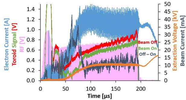
Figure 6: Initial beam commissioning. Axis label colouring denotes measurement type. Beam current is difference between toroid signals when extractor off and on.
