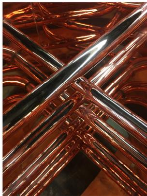
Figure 5: Third iteration of copper plating on Dummy 1 with the best result.
