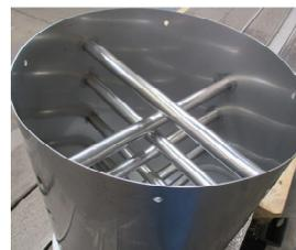
Figure 3: Dummy 1 consists of a simple rolled steel sheet with straight stems tacked inside.
