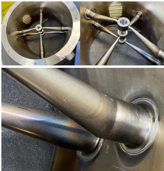
Figure 9: Dummy 4 – Pretest tank of CCH1 with three angular stems out of 3d-printed steel.
