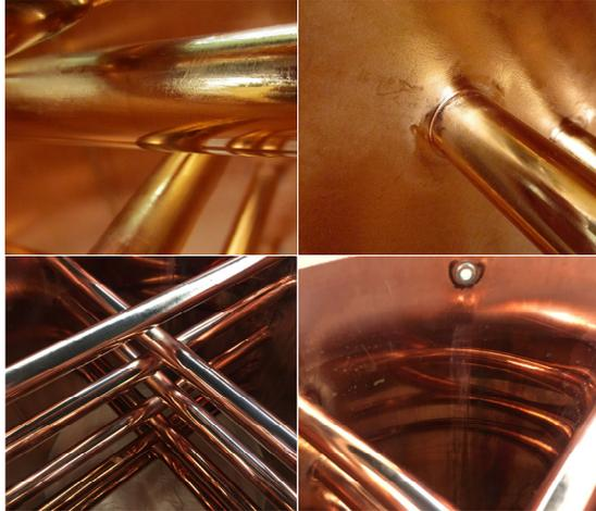
Figure 4: First copper plating iteration on Dummy 1 (top) and second iteration of copper plating (bottom).
