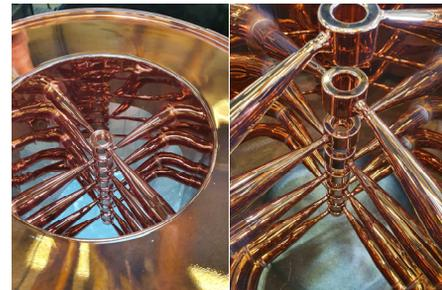
Figure 7: Copper plated Dummy 2 of CCH1.
