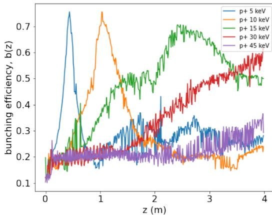
Figure 5: Bunching efficiency as a function of distance from the buncher center, for ESS-Bilbao proton beam with different extraction voltages.
