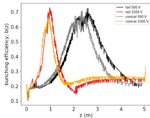
Figure 3: Bunching efficiency as a function of  $z$  for different geometries and electrode voltage, for HIE-ISOLDE beam.
