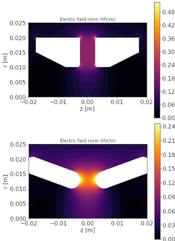
Figure 2: Electric field maps for the axisymmetric models with tail shape (top) and conical (bottom) buncher electrodes. Voltage between electrodes is 1 kV in both cases
