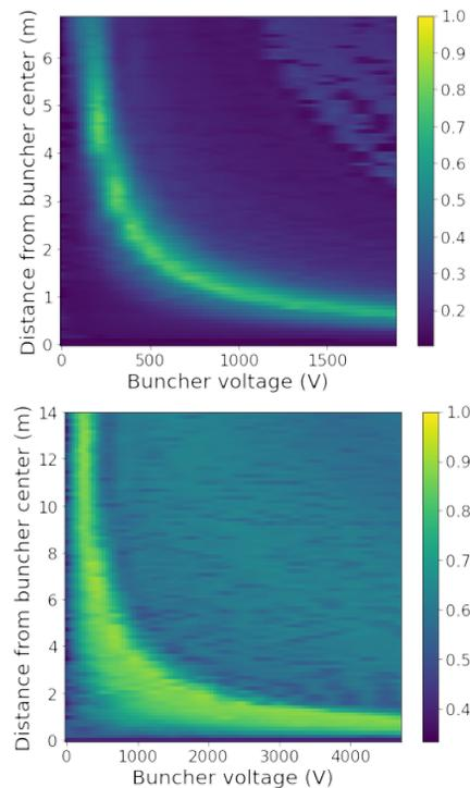
Figure 6: Heat map of bunching efficiency as a function of distance from the buncher center and electrode voltage, for ESS-Bilbao proton beam at 10 keV (top) and at an RF frequency of 35.2 MHz and 45 keV (bottom).
