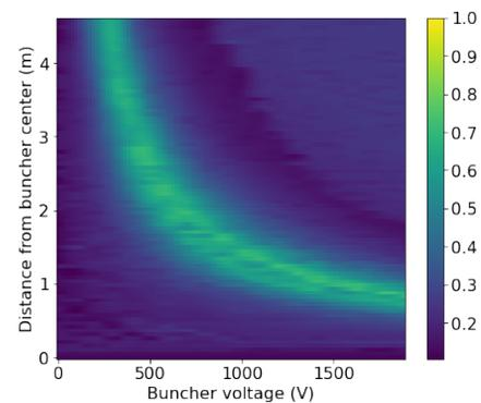
Figure 4: Heat map of bunching efficiency as function of electrode voltage and focal length, for ISOLDE beam.
