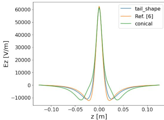
Figure 1: Comparison of on-axis field profile,  $E_z(z)$ , for three basic MHB geometries.
