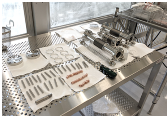
Figure 5: Edge welded bellows weldments and hardware in ISO 10 cleanroom after wet cleaning
