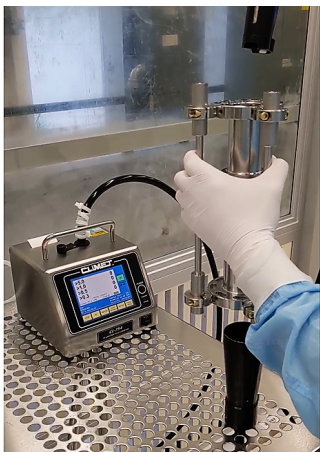
Figure 4: Edge welded bellows weldment dry blowing in ISO 10 cleanroom with filtered nitrogen
