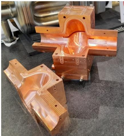
Figure 6: First 1.3 GHz SWELL cavity machined.
