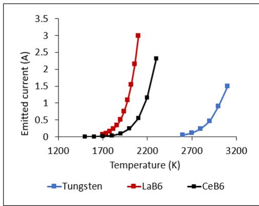
Figure 2: Maximum current emitted by cathode materials at given temperature.
