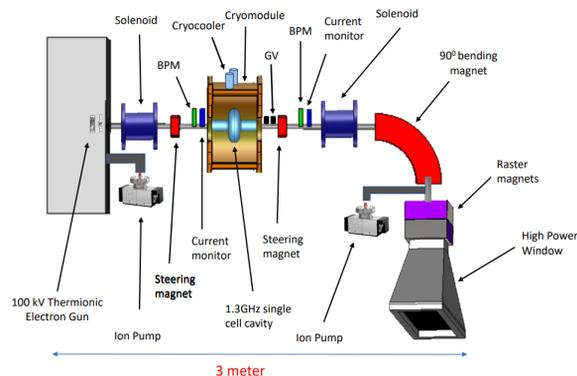
Figure 1: Schematic of proposed high-intensity, compact super-conducting linear electron accelerator.
