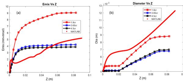
Figure 7: (a) Transverse emittance and (b) diameter comparison of the beam along bunch propagation direction ( $z$ ).
