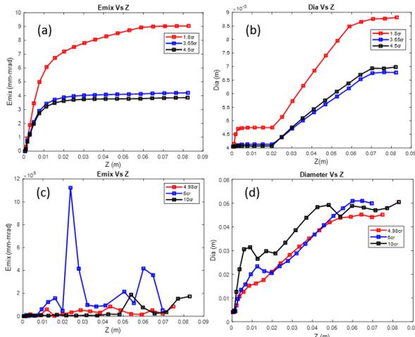
Figure 6: (a) Transverse emittance and (b) diameter variation of the beam with mesh density  $1.8, 3.65$  and  $4.5 \times 10^7$ , (c) transverse emittance and (d) diameter variation of the beam with mesh density  $4.98, 6$  and  $10 \times 10^7$  along bunch propagation direction ( $z$ ).
