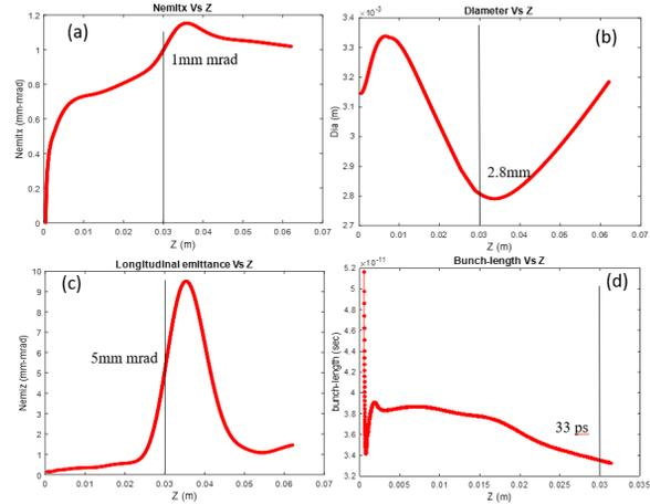
Figure 8: (a) Transverse emittance, (b) diameter (c) longitudinal emittance and (d) bunch-length variation along bunch propagation direction ( $z$ ).
