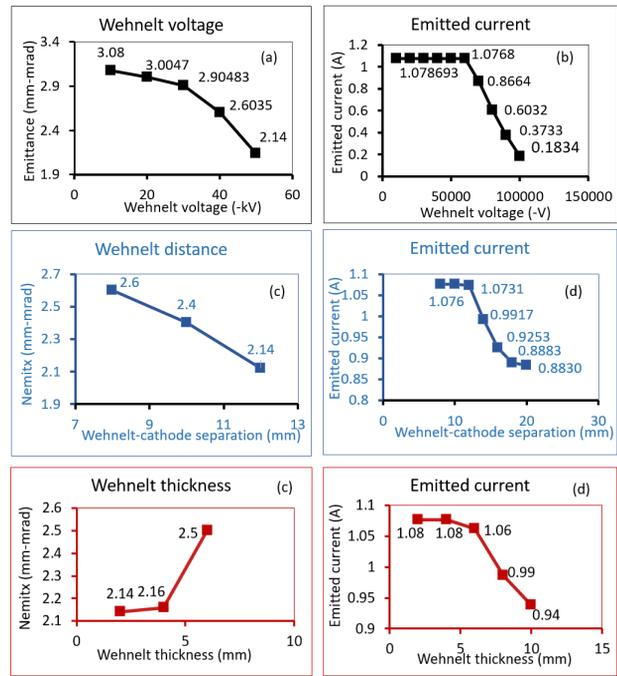
Figure 4: (a) Transverse emittance and (b) current variation with Wehnelt voltage, (c) Transverse emittance and (d) current variation with cathode-Wehnelt separation, (e) Transverse emittance and (f) current variation with Wehnelt thickness.
