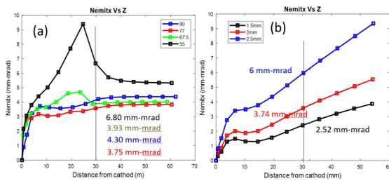
Figure 3: (a) Transverse emittance variation with angle of inclination of focusing electrode, (b) emittance variation due to cathode radius along bunch propagation direction (z).
