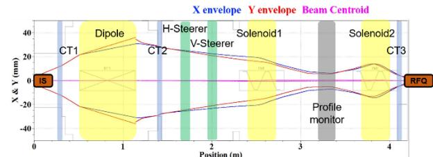
Figure 1: Layout and calculated beam dynamics of proton injector test stand at the KOMAC.
