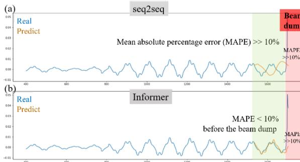
Figure 5: Comparison of the prediction models for beam orbit on a horizontal plane - (a) seq2seq (b) Informer.
