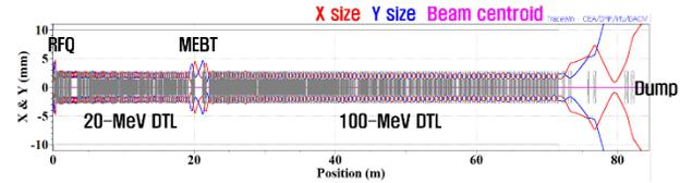
Figure 3: Calculated beam dynamics from 3-MeV RFQ to 100-MeV proton beam dump.
