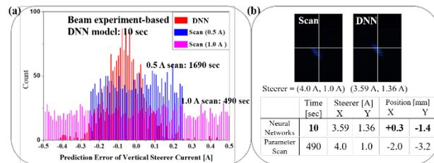
Figure 4: Comparison of prediction errors and consumed time between the DNN model and parameter scan method.
