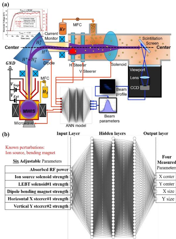
Figure 2: (a) Overview of beam experiments and flow of data to train deep neural networks model. (b) Layout of neural networks model for the low energy beam orbit correction.
