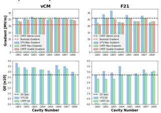
Figure 3: Gradient and Q0 comparison between VTS and CMTF tests for the vCM and F21.
