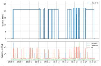
Figure 2: MP Processing – Cavity gradient (above) and radiation (below). Here one can see a quench followed by a stable run for approximately 2hr before repetitive quenching and processing.
