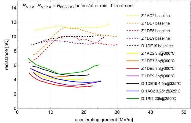
Figure 5:  $R_{BCS}$  estimation for all mid-T treatments and corresponding baseline measurements (dashed). “Z” stands for treatments at Zanon, while “D” abbreviates DESY. Temperature and duration of the treatments are given.
