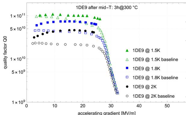
Figure 1: 1DE9 before and after mid-T treatment at Zanon with caps, no low T treatment was applied beforehand, hence the high-field  $Q_0$ -slope is visible in the baseline.
