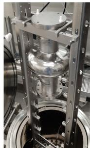
Figure 2: Single-cell cavity with DESY cap mounted on the insert of the niobium-retort furnace (visible at the bottom).
