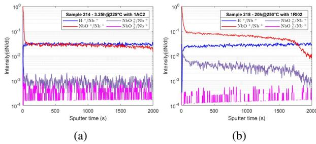
Figure 3: Normalised SIMS profiles for witness samples of (a) 1AC2 (3.25h@325 °C) and (b) 1RI2 (20h@250 °C). Shown are intensity vs. sputter time.
