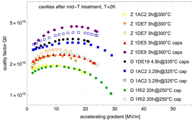
Figure 4:  $Q(E)$  for all mid-T treatments. “Z” stands for treatments at Zanon, while “D” abbreviates DESY. Temperature and duration of the treatments are given and whether the cavity was closed by caps. Empty markers depict curves, which were stopped before reaching the quench.
