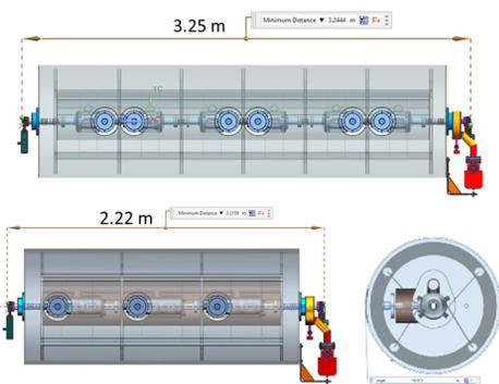
Figure 4: Conceptual cryomodule layout for 1-cell (top) and 2-cell (bottom left) cavity options with front view (bottom right).
