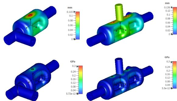
Figure 11: Deformation (top) and stresses (bottom) for the 1-cell (left) and 2-cell (right) cavities at the maximum tuning range.
