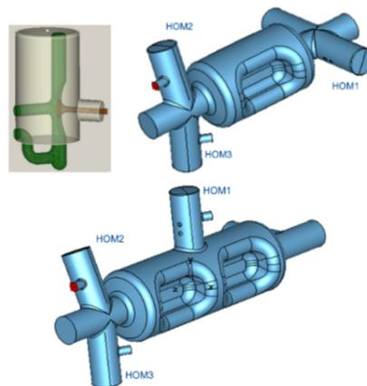
Figure 6: TESLA HOM coupler (top left), 1-cell cavity with HOM dampers (top right), and 2-cell cavity with HOM dampers (bottom).
