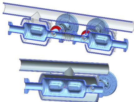
Figure 5: Conceptual He vessel layout for 1-cell (top) and 2-cell (bottom left) cavity options.
