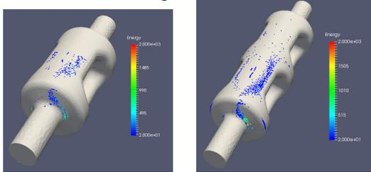
Figure 8: Multipacting resonances of the 1-cell (top) and 2-cell (bottom) cavities.
