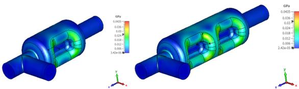
Figure 10: Stresses in the 1-cell (left) and 2-cell (right) cavities at an external pressure of 2.2 atm.
