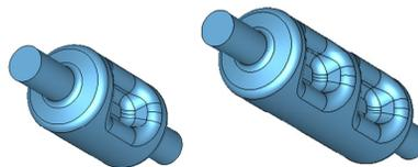
Figure 3: 1-cell (left) and 2-cell (right) 1.3 GHz rf-dipole crabbing cavities.
