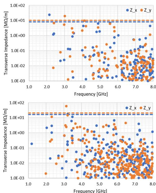
Figure 7: Horizontal and vertical impedances for 1-cell (top) and 2-cell (bottom) cavities.
