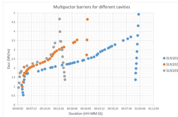
Figure 3: Time to condition the multipactor barriers for 3 LB cavities.
