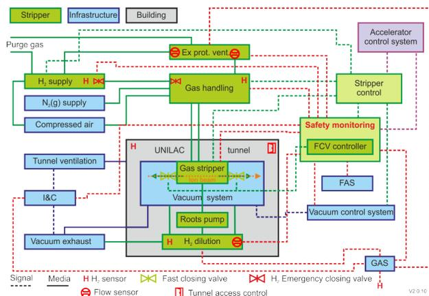
Figure 2: Simplified schematic overview of the current gas stripper system design. Green: specific parts of the gas stripper system, red: safety devices, blue: common infrastructure, violet: accelerator control system, grey: UNILAC accelerator tunnel building.
