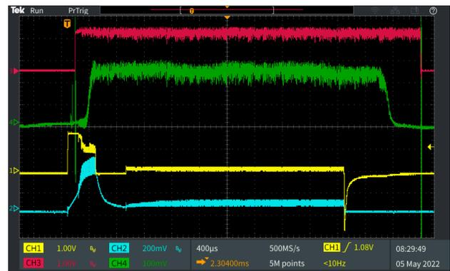
Figure 3: Oscilloscope screenshot showing the stripping of  $\text{Ar}^{2+}$  ions with the pulsed gas stripper using  $\text{H}_2$  as stripping target. Shown are the current of the incoming beam (red) and the stripped  $\text{Ar}^{12+}$  beam (green), as well as the voltage (yellow) and current (cyan) applied to the valve.
