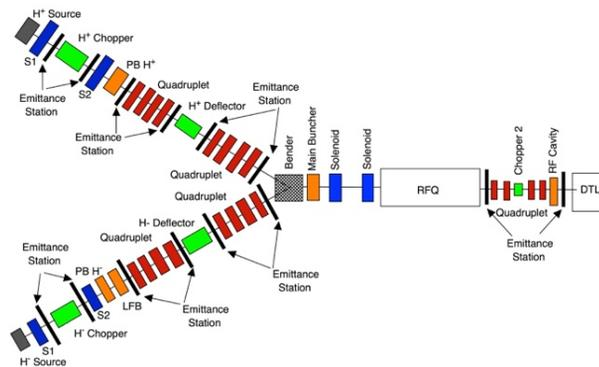
Figure 1: Layout of proposed RFQ-based 3-MeV injector.
