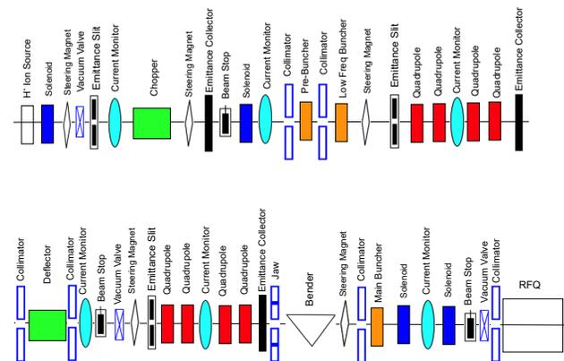
Figure 2: Layout of H<sup>-</sup> leg of injector part with additional beamline elements.
