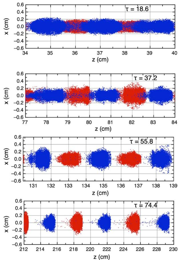
Figure 5: Formation of the two-component beam in RFQ: (red) H<sup>+</sup> beam, (blue) H<sup>-</sup> beam; numbers indicate RF periods  $\tau = tf$ .
