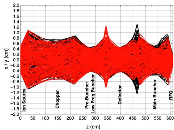
Figure 3: Particle trajectories in the injector beamline: (red) horizontal, (black) vertical.
