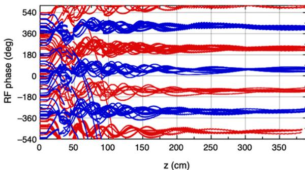
Figure 4: Phase trajectories in two-component beam in RFQ: (red) H<sup>+</sup> beam, (blue) H<sup>-</sup> beam.
