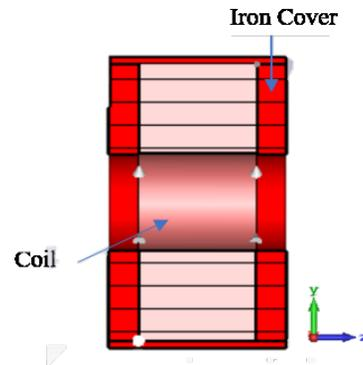
Figure 4: A schematic view of solenoid.
