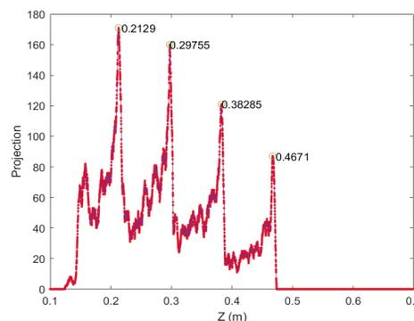
Figure 9: Beam projection after ejected from the buncher (every peak represent a bunch).
