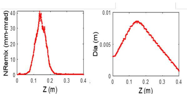
Figure 7: Change in normalized RMS transverse emittance (left) and beam diameter (right) with direction of propagation.
