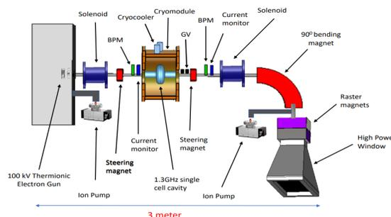
Figure 1: Schematic of proposed accelerator.
