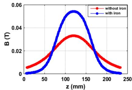
Figure 5: Magnetic field with and without iron cover.
