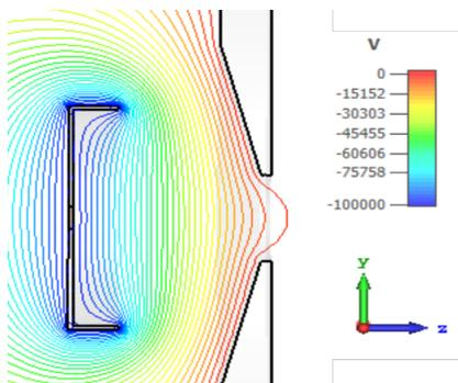
Figure 3: Equipotential lines generated due to the applied potential of -100 kV on cathode.
