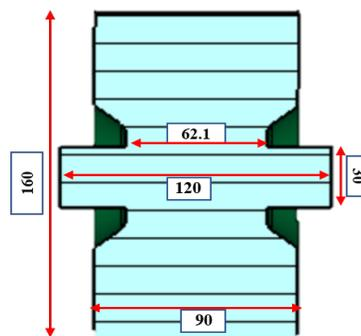
Figure 8: Cross sectional view of buncher cavity (units in mm).
