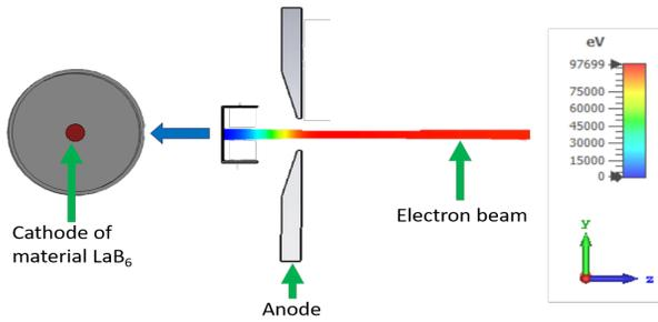
Figure 2: Cross-sectional view of the electron gun.
