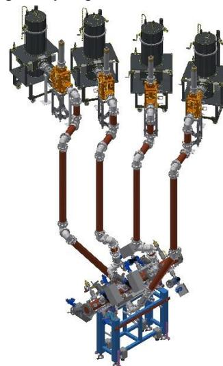
Figure 2: 3D model of 750MHz coaxial lines
