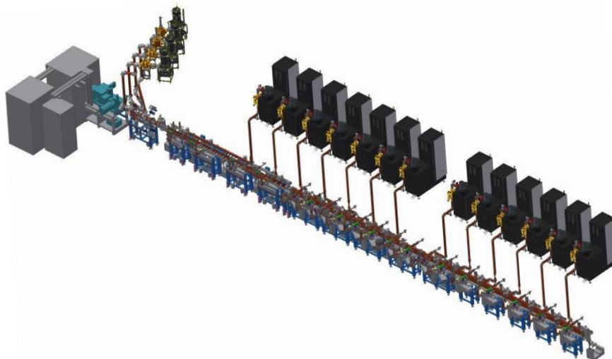
Figure 1: 3D model of the full LIGHT. The 3 GHz RF Network is visible connecting the high power stations to the accelerator.
