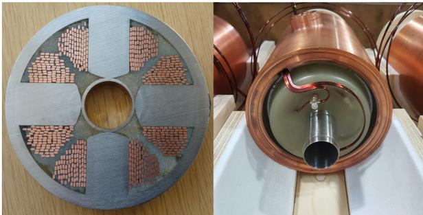
Figure 2: A section of a proto-type magnet (left); a magnet and beam tube assembly in a drift tube body (right).
