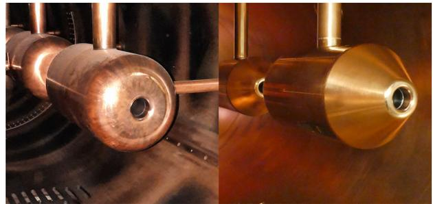
Figure 3: The old (left) and new (right) drift tube shapes. Note the vacuum patch just visible in the background of the left hand image.
