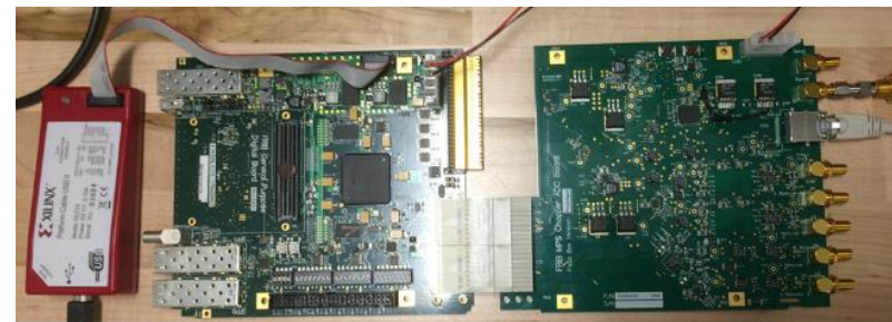
FGPDB and high speed ADC board developed
