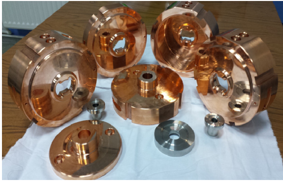
Before brazing, manufactured CANDLE SRI, Yerevan
