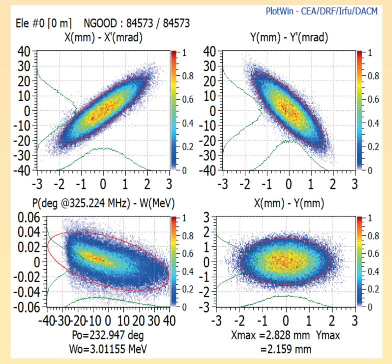
Figure 3: Phase-space plots and distribution projections (green curves) at the RFQ exit (10 mm behind the electrode ends) in the case of an entrance current of 100 mA. The colors of the scatter plots refer to the normalized (macro) particle density (linear scales at the right frames of the plots). The red ellipses correspond to the 95% emittances.
